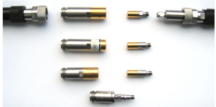
Figure 12: Calibration standards and adapters for a noninsertable device
